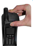
2. Push EJECT and phone at the same time
